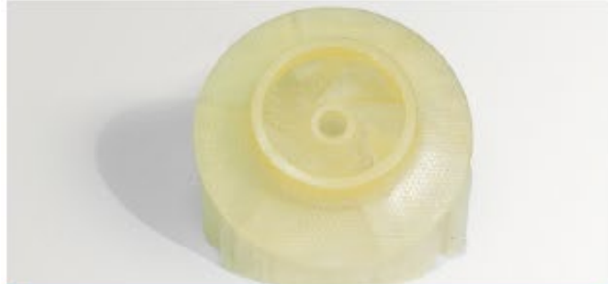
Pump Rotor Core Investment Casting
